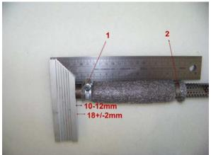
Clamp (1) must be fitted at a distance of 18+/-2mm, measured from the end of the tube.
