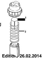
c) The tolerance gauge (ROTAX part no. 277 400) must **not** be able to turn around (opening limit of carburetor slide)!
